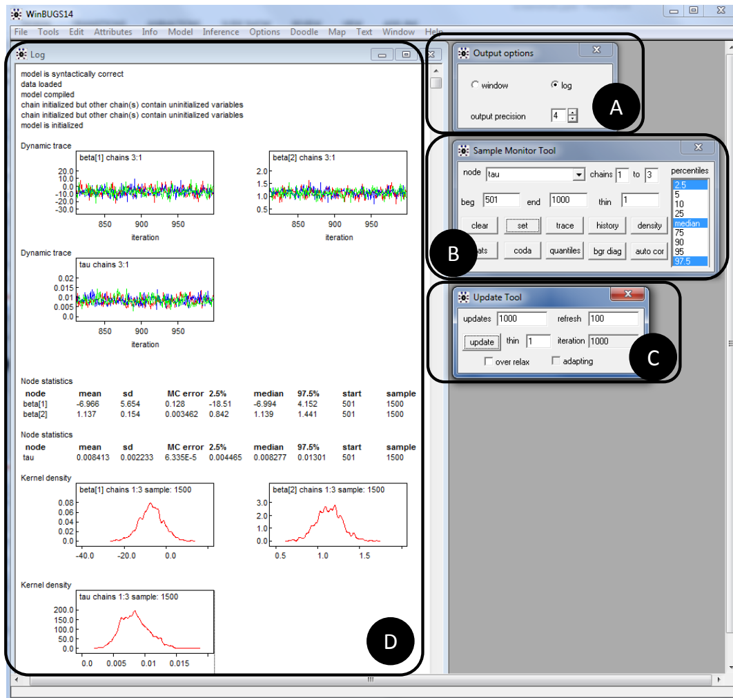
Figure 2. The WinBUGS graphical user interface continued. Panel A shows the Output Options window; Panel B shows the Sample Monitor Tool window; Panel C shows the Update Tool window; Panel D shows the log file.
